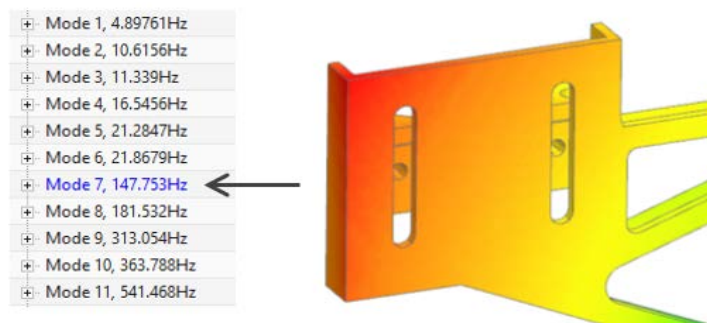
Analysis 1: Simulation of structural dynamics - Mode 7 is identified as component resonance at 147.8 Hz.
